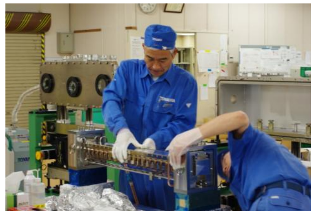
Engineers assembling a mirror bender system
