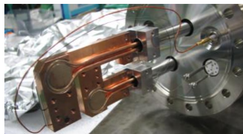
Cooled slit with current and temperature monitoring
